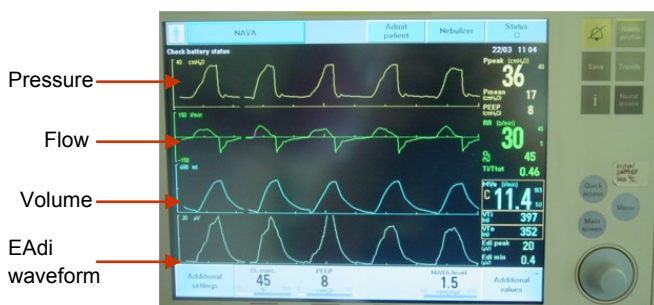
Figure 3: The EAdi waveform should be displayed on the monitor screen of a ventilator during NAVA.
