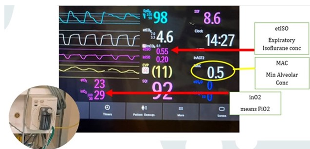
Fig. 4 EtISO, MAC and inO 2 Values from Gas Analyzer as shown in a Patient Monitoring System
